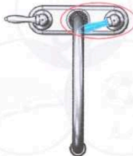
Collision Detection with Stop at collision active. Notice the handle cannot move inside the faucet.
