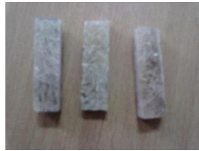
Fig:16 Specimen used for Water absorption and chemical corrosion test
